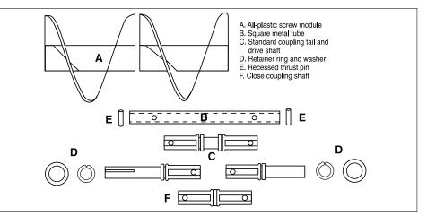
The Martin screw conveyor system consists of plastic modules stacked on a square metal tube. A shaft is inserted at each tube end and secured by a recessed pin. Modules are secured at tube ends by retainer rings and washers.
